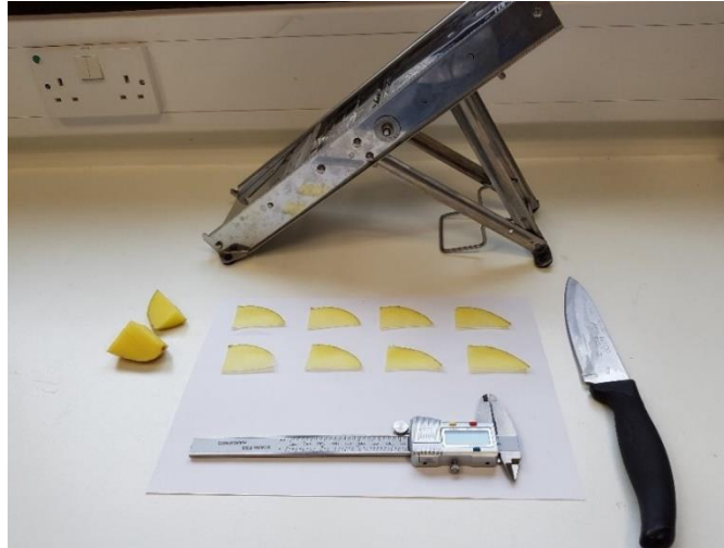
Figure 2-1. Tools used to slice potato tubers and measure slice thickness during fry colour study.
