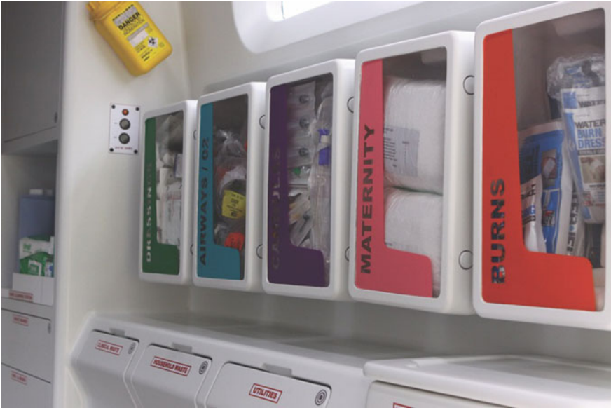
Fig. 11 Treatment packs that can be replaced at the end of each shift reduce restocking time and complexity
