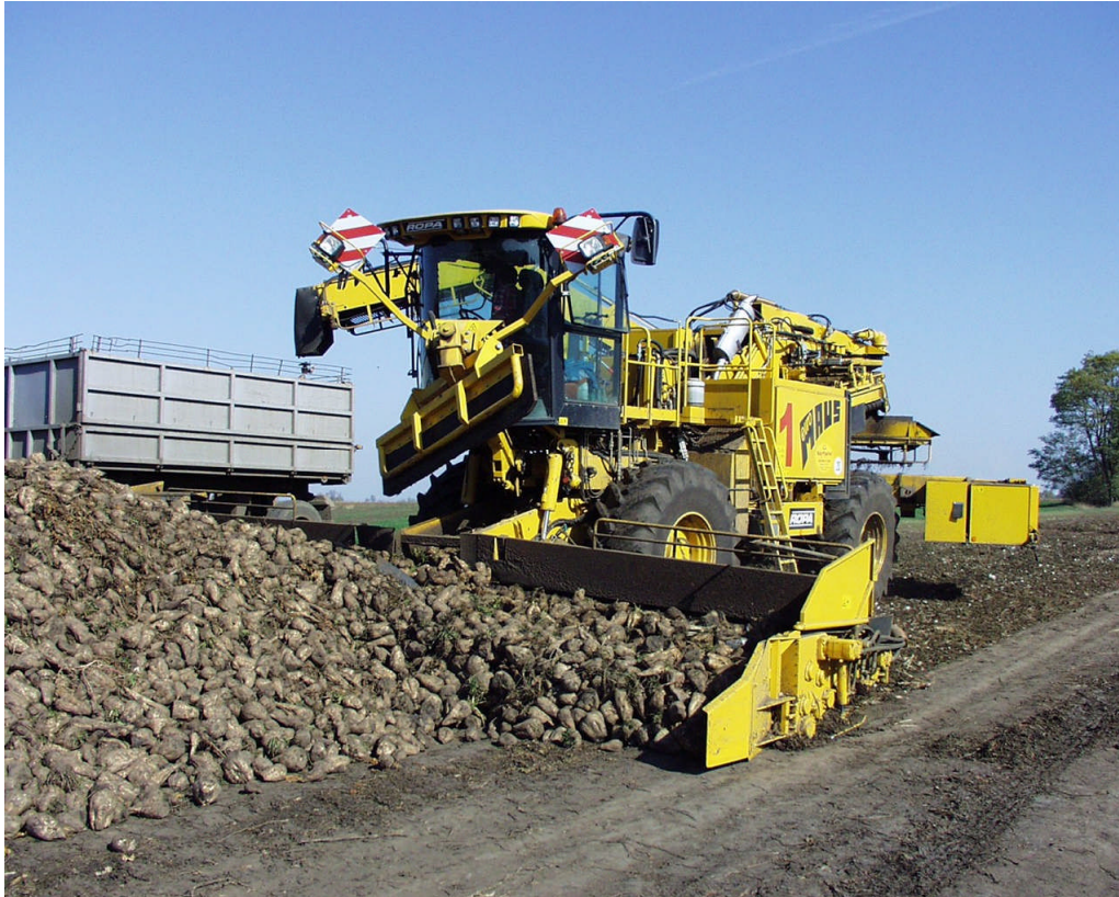
Fig. 2. Cleaning and loading machine in operation
