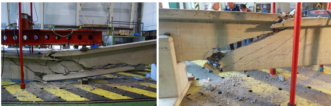
Fig. 3 Bending (left) and shear (right) failure
