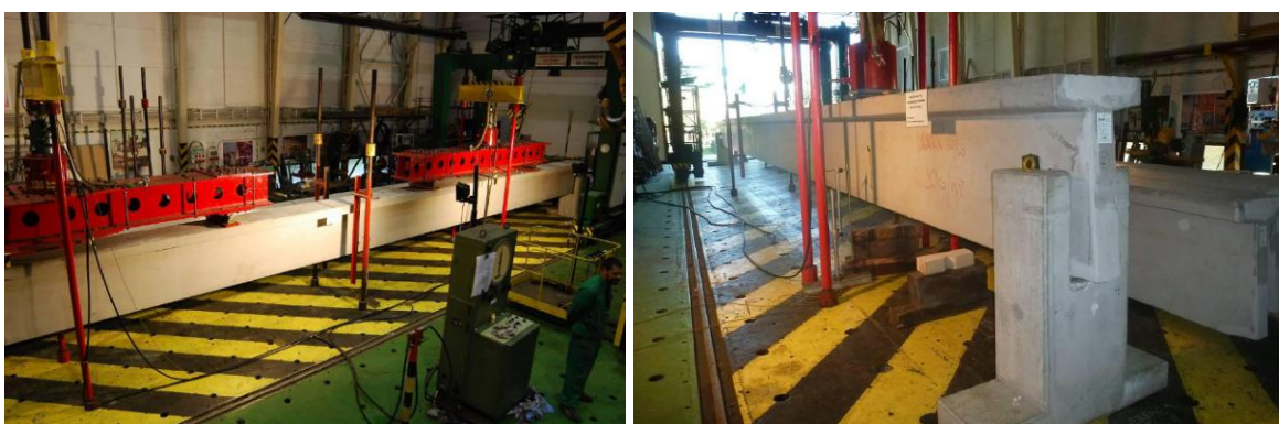
Fig. 2 Bending (left) and shear (right) tests
