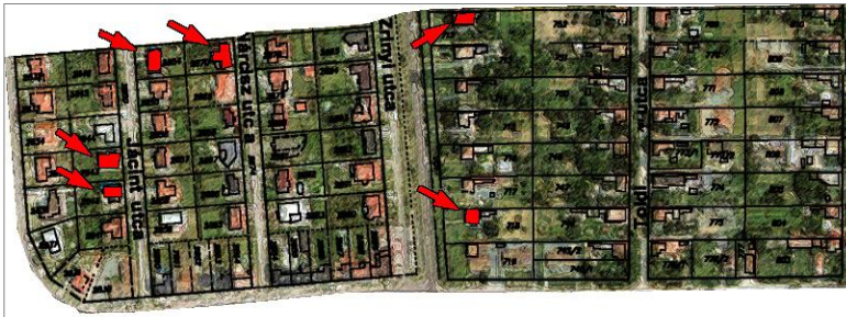
Fig. 2. Different hue of the roofs on test area for supervised classification. Note that if roofs are deselected based on one pixel intensity, certain roofs are not deselected, denoted with red arrows
