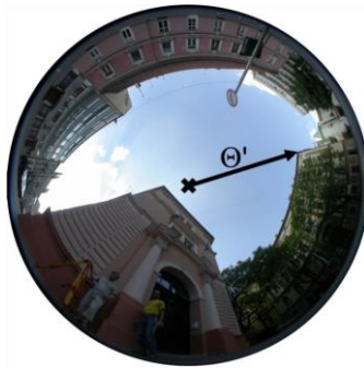
Fig. 7 Example of a fish eye photograph. x = center of the image, arrow and \Theta' = distance between image's center and obstacle
