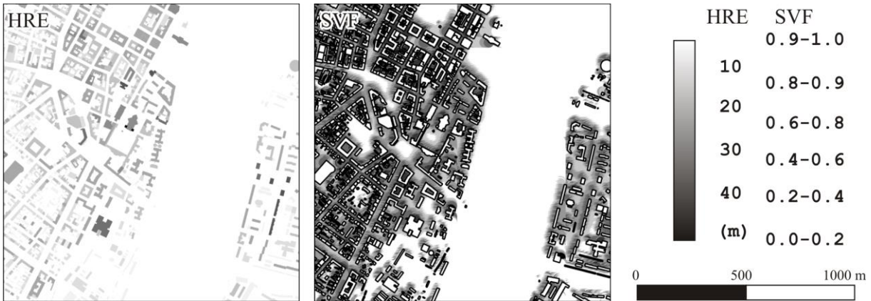
7 8 Fig. 5. Patterns of building height and sky view factor in a selected part of the study area as 9 examples 10 11 12 13
