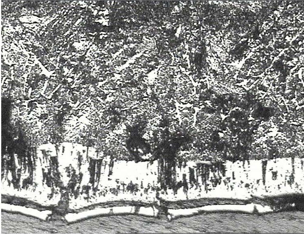
Fig. 62. Spalling oxide scale on rod No. 1 at 350 mm elevation
