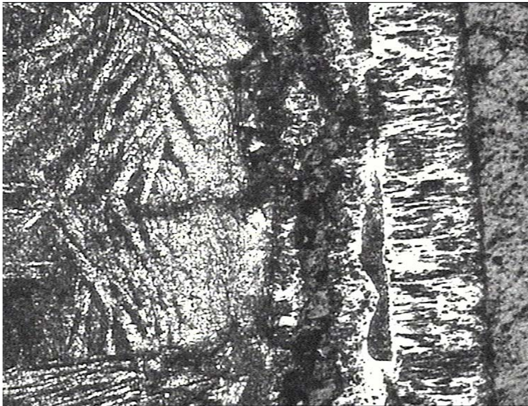
Fig. 65. Internal oxide scale on the shroud at 750 mm elevation
