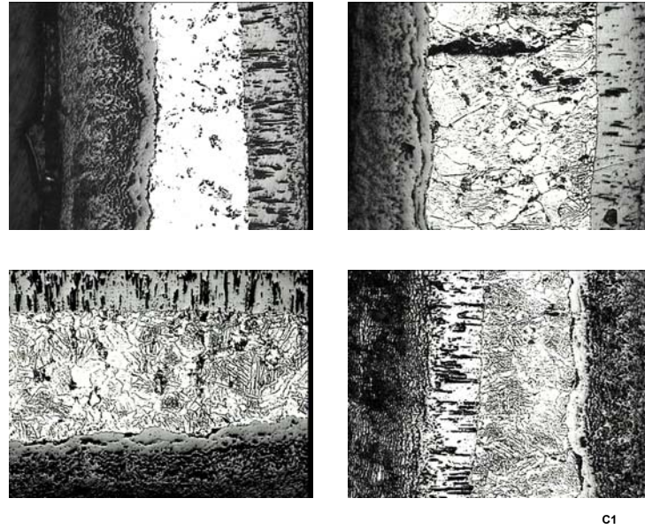
Fig. 75. Cross sections of cladding tubes of the preliminary test (central section)
