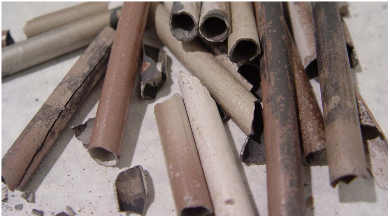
Fig. 69. View of the broken cladding tubes CODEX-CT preliminary test
