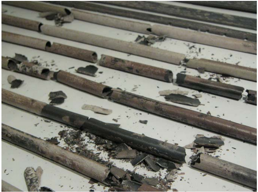
Fig. 68. View of Zr cladding and shroud plates after the CODEX-CT preliminary test
