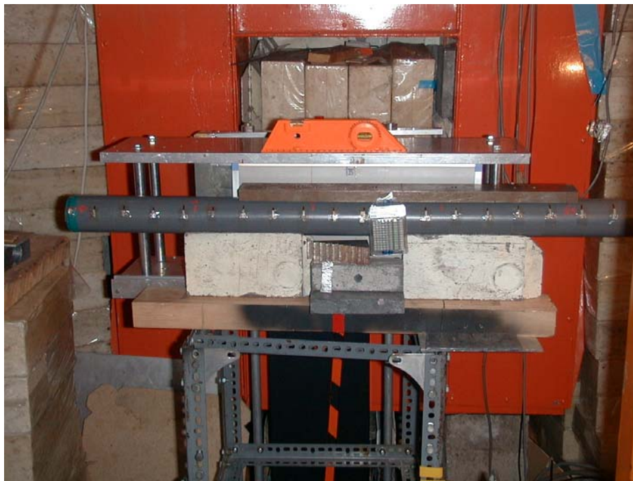
Fig. 79. X-Ray radiographic examination of the CODEX-CT-1 bundle (the bundle is inside of the horizontal plastic tube in the exposure position)
