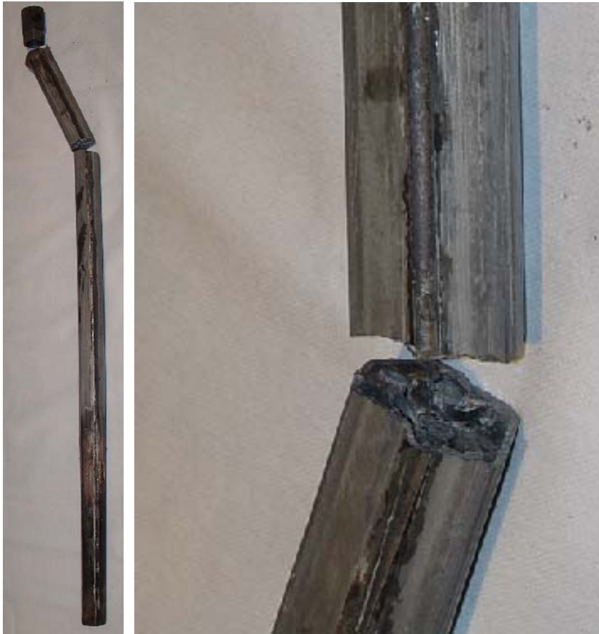
Fig. 78. View of the CODEX-CT-1 bundle after the experiment (left) and close view of the broken cross section (right)
