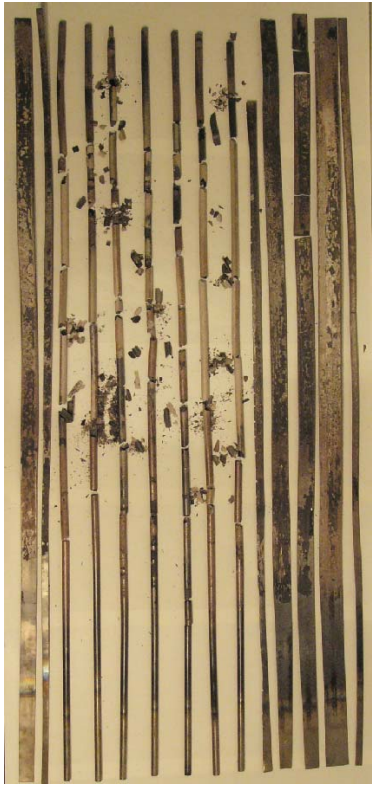
Fig. 68. View of Zr cladding and shroud plates after the CODEX-CT preliminary test
