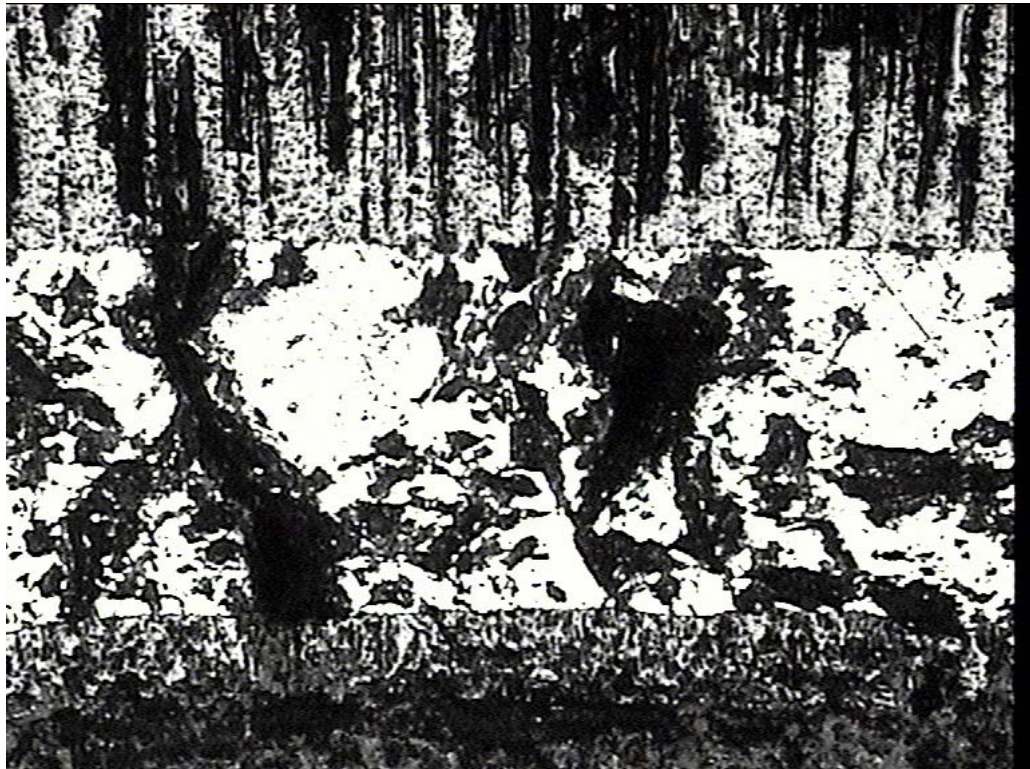
Fig. 86. Rod No. 1 at 710 mm elevation with external (top) and internal (bottom) oxide scales
