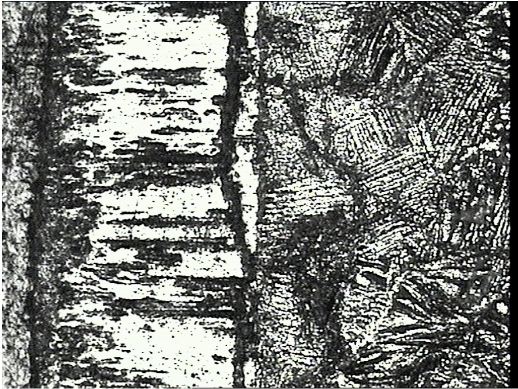
Fig. 87. Oxide scale on the shroud at 810 mm elevation
