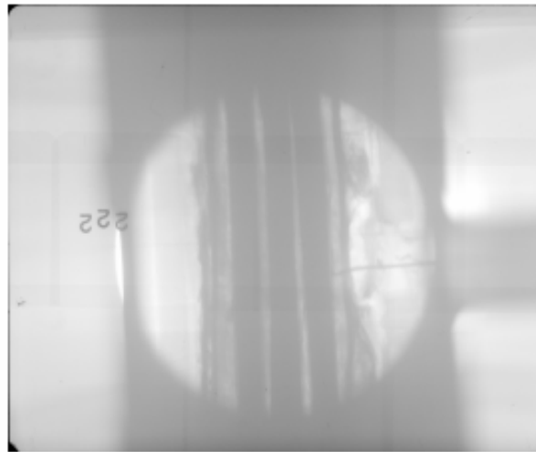
Fig. 96 X-ray radiography view of the upper part of the CODEX-B4C bundle at ~465 mm elevation (pictures taken at 17000 s, 20400 s and after the test)
