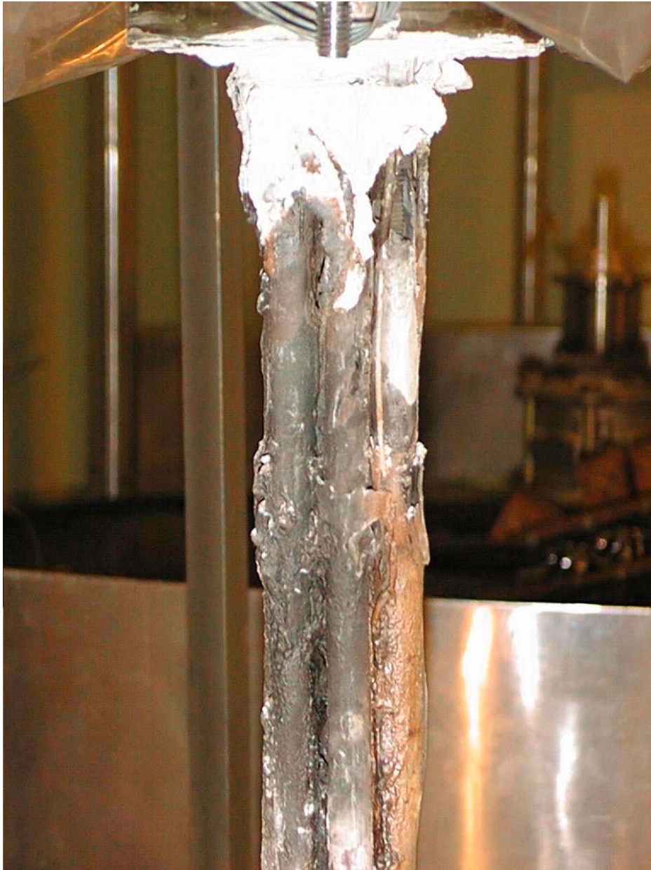
Fig. 90 View of the upper part of the CODEX-B4C bundle
