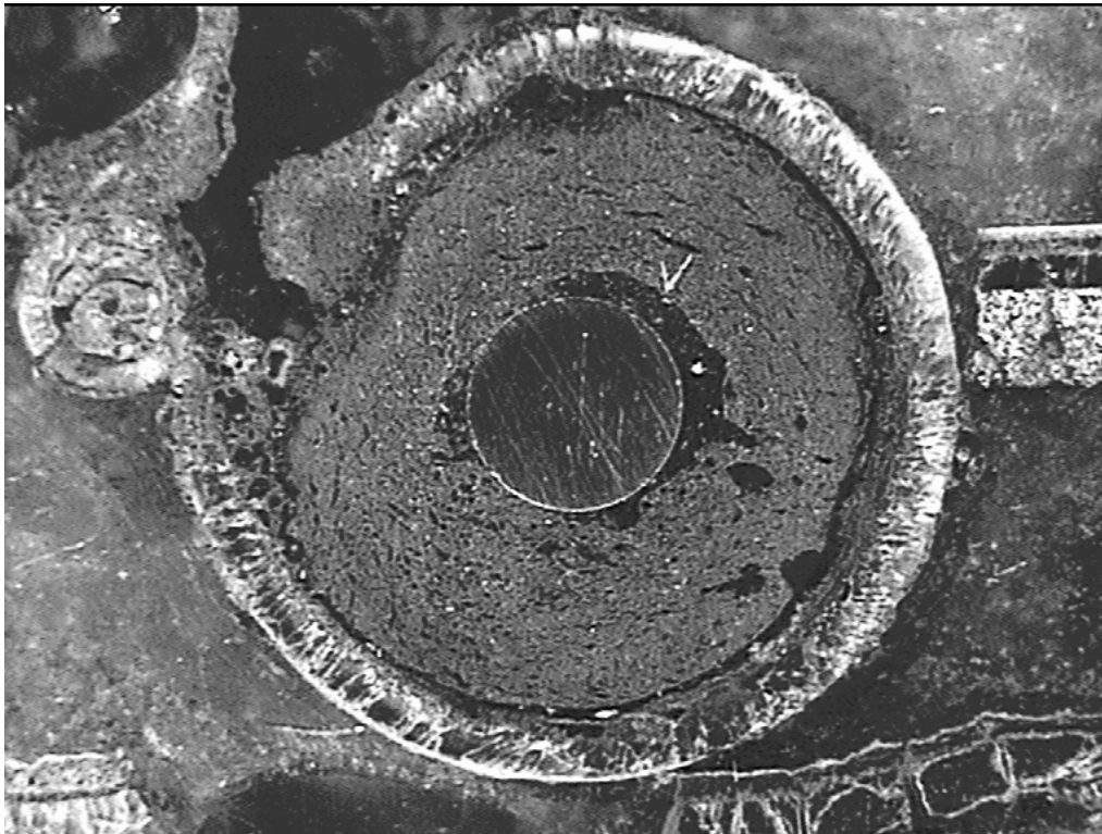
Fig. 109 Chemical interactions between cladding, pellet and thermocouple inlet metal shielding at 555 mm elevation
