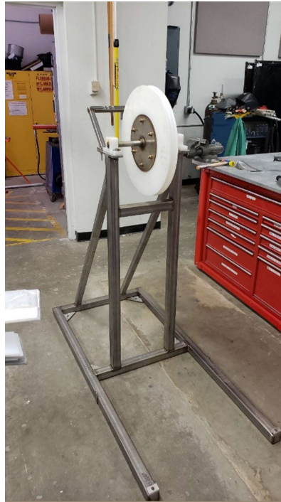
Figure 44. Completed Sheave Holder Assembly.
