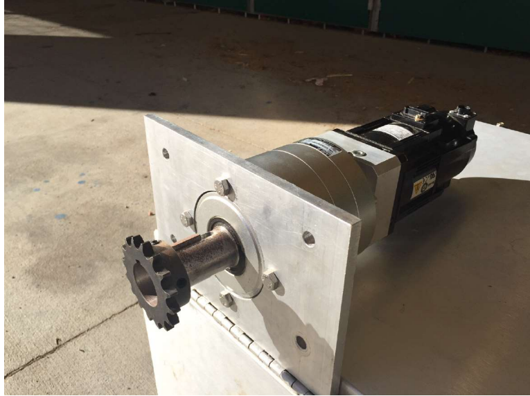
Figure 20. Yaskawa ServoPak and planetary gear reducer (Nelson, Miller, Maalouf, & Shah, 2015).
