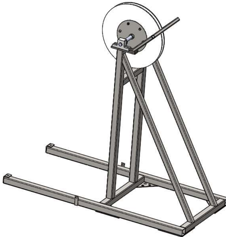
Figure 18. CAD design of sheave holder.
