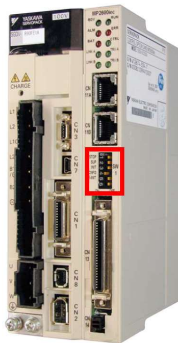
Figure 24. Configuration DIP switches on ServoPak PLC. (Yaskawa, 2018).
