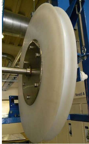
Figure 17. Original Delrin sheave designed by first Pier Portal group. (Belis, et al., 2012).
