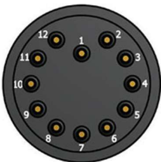
Figure 38. Pin numbering scheme for the SubConn 12-contact underwater connector.
