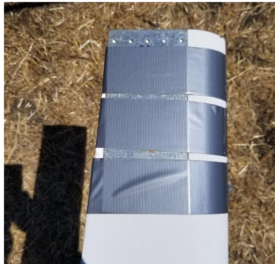
Figure 3.1: Test setup of 100g mass imbalance. The mass is attached to the downwind, “suction” side of the blade.
