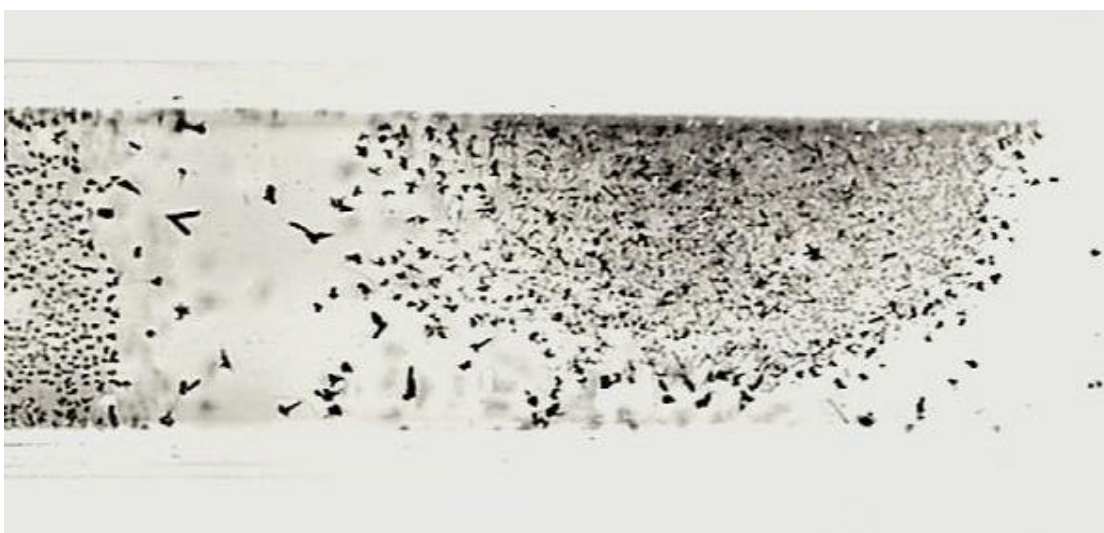
Figure 33. RuO 2 crystals inside an inlet quartz tube.
