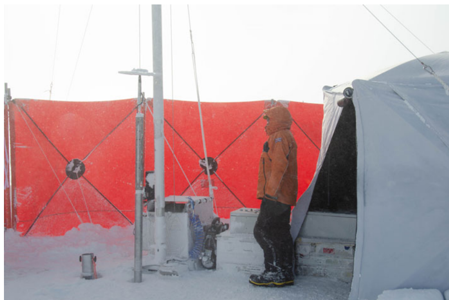
Fig. 13. BAS-RAID drill (Rix and others, 2019) in action in bad weather on Sherman Island. The winch and mast are central in the picture, with the drill exiting from the borehole; only the anti-torque section and the motor-controller section are visible. To the right is the temporary pop-up shelter for the drill controls. Pop-up windbreaks protect the driller, standing in front of the winch control panel, from the wind and drifting snow. To the left, the top of the sampler tube is visible projecting from a vertical hole in the snow, designed to enable filling, and to keep the sampler chilled between runs to avoid chips sticking in its barrel.
