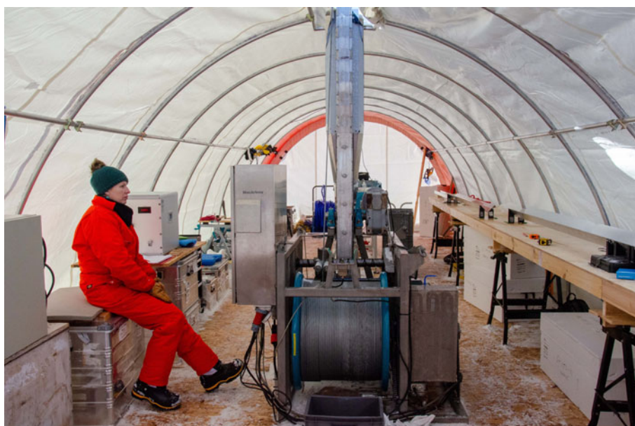
Fig. 7. Drill infrastructure in the Weatherhaven shelter. The winch and mast dominate the foreground, with the drill operator sitting to the left. On the right is the core processing table.
