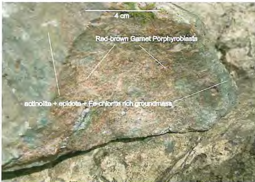
Figure 3.12. Red-brown cross-cutting garnet mineralization in actinolite + epidote altered basalt in the Central Basalt Sequence. 4 cm bar for scale. Outcrop 087.
