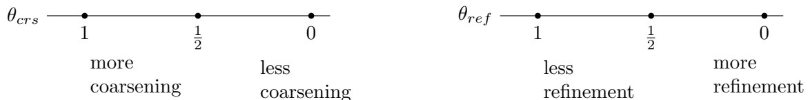
Figure 8: Sketch of influence of grid parameters \theta_{crs} and \theta_{ref} on the mesh manipulation process.
