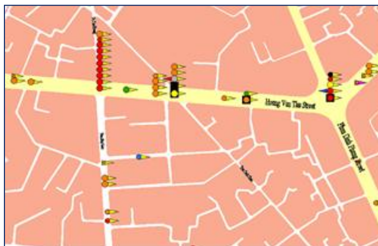
Figure 10. Typical example of Accident Pin Board (APB) of the area under study
