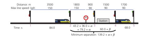
Figure 2. Capacity calculation
