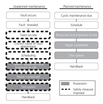
Figure 4. Maintenance tasks during unplanned and planned maintenance
