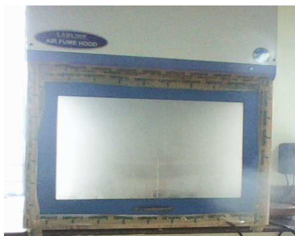
Fig 6: Modified mosquito bioassay chamber -Fume hood filled with smoke after fumigation with Aparajitha dhooma choornam
