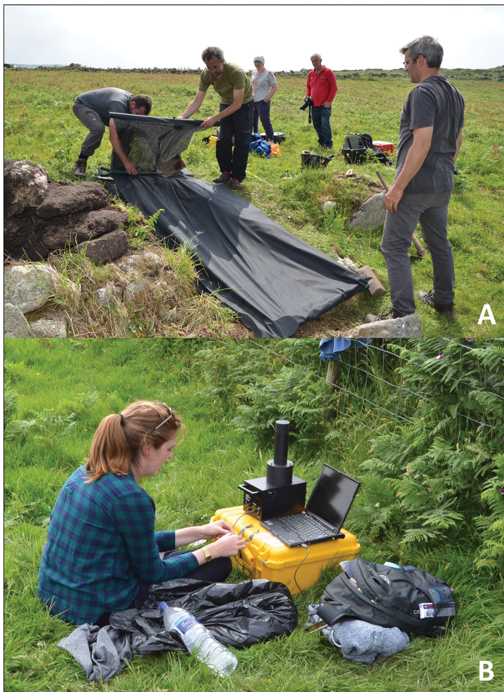
Figure 3. Site 1 being protected from light under a dark cover (A), and analysis of soil samples using the portable OSL reader (B) (photographs by S. Vervust).
