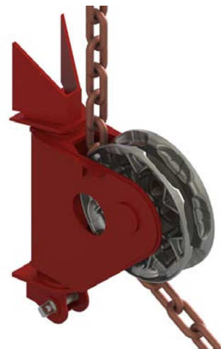
Figure 2. Sketch of mooring chain wheel at fairlead [11]
