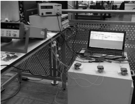
Fig. 11. Experimental setup for testing single tooth ISG windings
