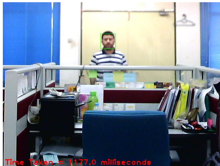
Figure 3.16: Searching for a face of size 20x20 can result in a speed of 0.85 FPS
