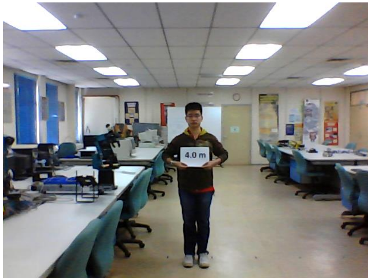
Figure 4.8: A subject holding a cue card and standing 4.0 meters away from the cameras
