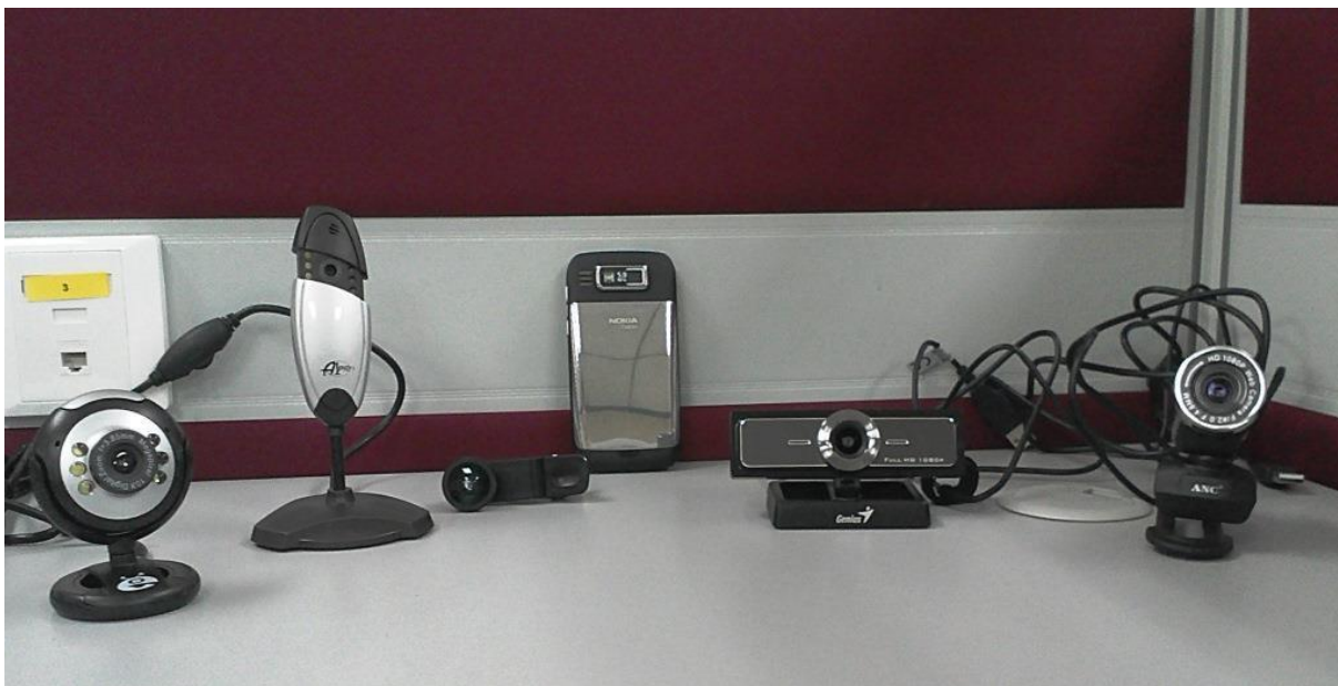
Figure 4.2: The camera's used in the experiment, from left to right: The slim webcam, the A1-Pro webcam, the fisheye lens, the E72, the Genius F100 and the Full-HD webcam
