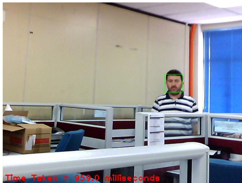
Figure 3.15: The time taken to scan for a face of size 25x25 pixels
