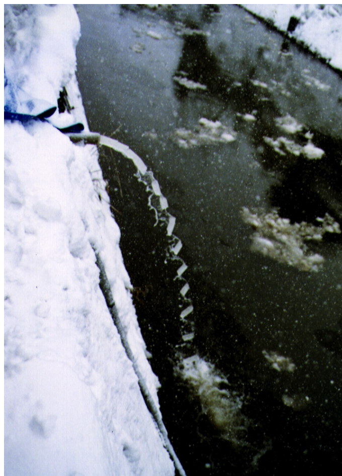
Figure 4. High snow fraction column flow of fresh-snow/water slurry discharging from pipe exit.
