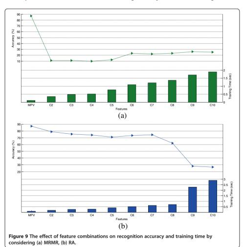
MPV. The main reason was that although some of the single features provided meaningful power for classifying the gestures individually, their combinations not only delivered less discriminative feature sets but also caused more data overlapping between the classes which reduced the classification accuracy.
