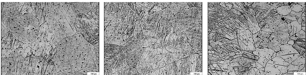
Fig. 3. Optical microstructure of Mg-1Ca binary alloy forged at the speed of 50 spm and sample temperatures of (a) 250, (b) 350 and (c) 450 °C
