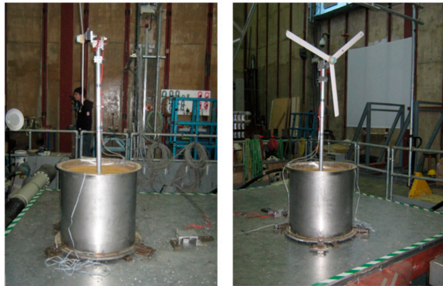
Figure 29. Illustration of the model wind turbine positioned on the BLADE shaking table.
