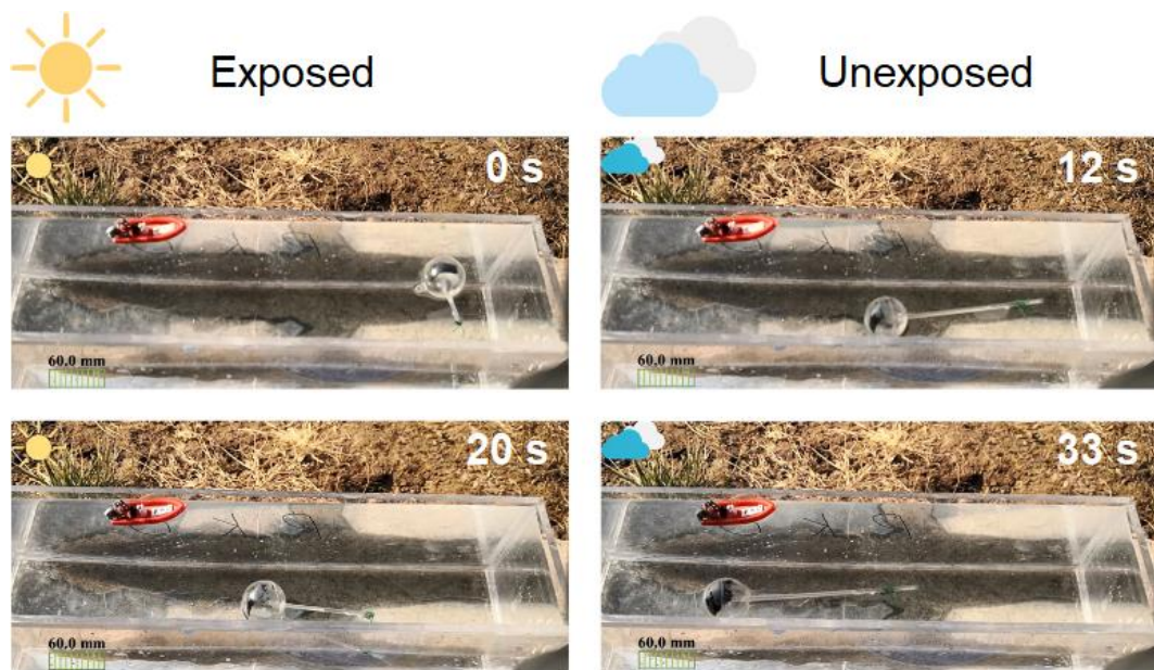
Fig. 4. Sunlight driving PPFR. Digital images showing a PPFR swimming, when it is exposed and unexposed to outdoor sunlight alternately. The average swimming speed achieves 9.6 \text{ mm s}^{-1} .
