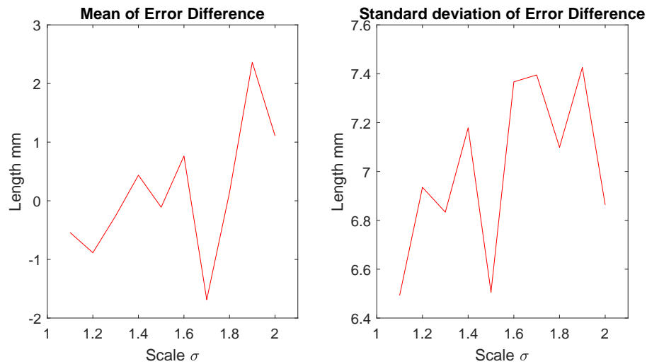
Figure 4.9: Mean (LEFT) and standard deviation (RIGHT) of the difference in arclength between original images minus the scaled images. The correlation coefficient of the mean and standard deviation against scale are r = 0.55 and r = 0.51 respectively.
