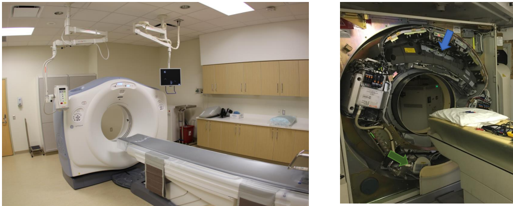
Figure 1.2: LEFT: A image of a CT scanner in a clinical setting. RIGHT: The internal components of the CT scanner. The X-ray tube (green arrow) and detectors (blue arrow) rotates as the patient transverse through the bore. Images adapted from Wikipedia, en.wikipedia.org/wiki/CT_scan , last accessed on May 4, 2021.
