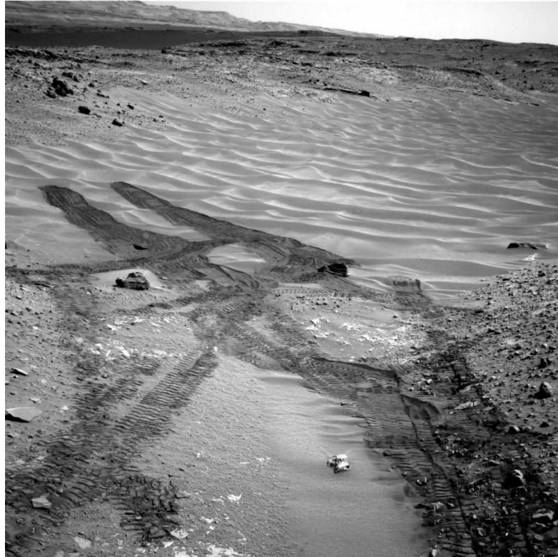
Fig. 1. The Hidden Valley on Mars ©NASA/JPL. Curiosity experienced excessive wheel slip here and failed to traverse this region although it is relatively flat. At the beginning of the mission, Curiosity was commanded to travel on the flat surface and avoid obstacles such as rocks; however, wheel slip occurred owing to loose sand with megaripples. Wheel traces on these megaripples indicated that Curiosity gave up traversing this surface and turned back to avoid getting stuck.
