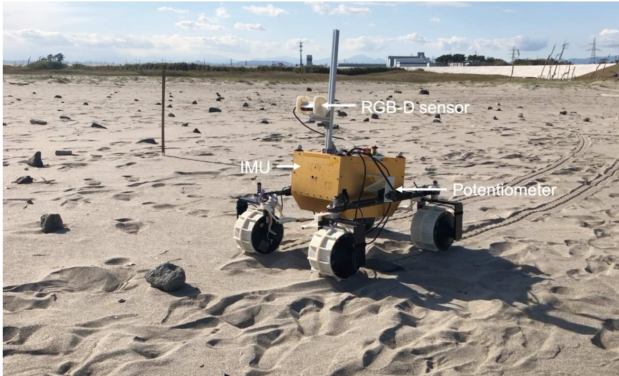
Fig. 7. El-Dorado IIB rover testbed on sandy terrain. RGB-D sensor, IMU inside the main body, and potentiometers attached to each side of the body are used for acquiring data.
