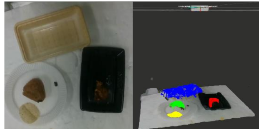
Fig.8 RGB frame of the depth camera (Left) and extracted point cloud visualization (Right).
