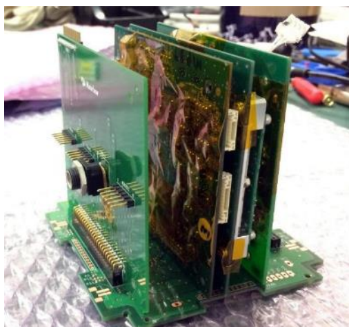
Figure 5. BIRDS-1 subsystem boards inserted on the prototype of SoftCIB
