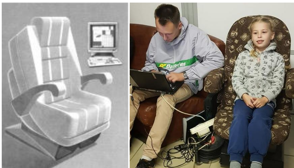
Figure 12: Chair containing the WBC and body measurements conducted by BELRAD institute in Minsk airport, July 13, 2019 (Osona amb els nens, 2019).
