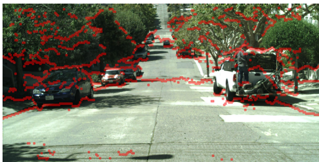
Fig. 9 Sample image from the real-data sequence used for Stixel cut generation. Stixel cut ground-truth is highlighted in red (Color figure online)
