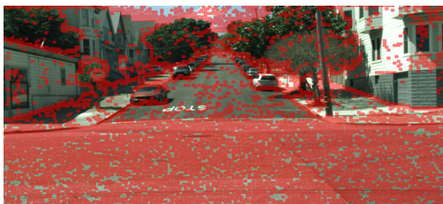
Fig. 6 Generated Stixel cuts (highlighted in red) using the left and right extrema as defined in Ignat (2016), and also cuts generated from semantic segmentation. Stixel cut density is 30%, equivalent to a 3.3× reduction in vertical resolution (Color figure online)
