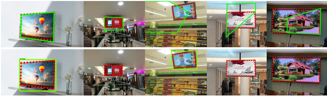
Figure 2: Screen extraction performance of (1st row): Edge analysis algorithm, and (2nd row): SSD-MobileNet, with photos of representative displays. The ground-truth borders are drawn in “dotted red” lines while the detected borders/bounding boxes are drawn in “solid green” lines.
