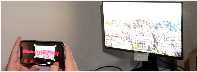
Figure 16: A smartphone, running DeepLight -enabled captioning application, displays the text (in ‘Alice in wonderland’ textbook) decoded from a monitor.
