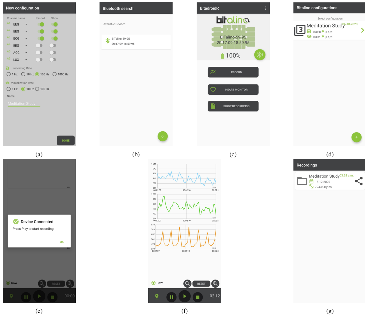
Figure 2.2: (a) Configuration of the acquisition parameters; (b) Search for Bluetooth devices and selection of device corresponding to BrainBIT; (c) The application interface in which to begin acquisition simply press the RECORD button; (d) Select the configuration to start the acquisition; (e) To start the acquisition press the PLAY button; (f) The EEG and PPG signals with a delay of 0.1 s; (g) The saved data from the acquisition.
