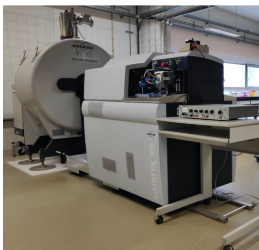
Figure 1.2. 7 T Solarix XR FT-ICR Mass Spectrometer present in Fourier-Transform Ion-Cyclotron-Resonance and Structural Mass Spectrometry Laboratory (FT-ICR-MS-Lisboa).
