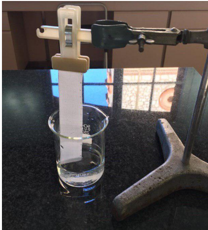
Figure 6.4. Vertical wicking test of PET/Co without impregnation
