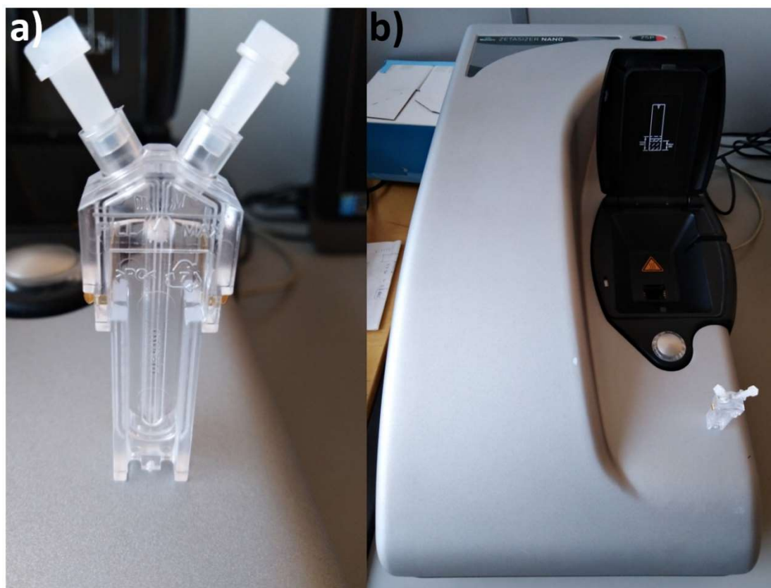
Figure 3.18. ZetaSizer Nano utilized in this work. a) Folded capillary cell for \zeta -potential and DLS measurements. b) ZetaSizer Nano.
