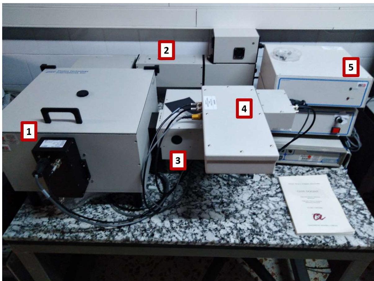
Figure 3.19. QuantaMaster 400 Photon Technology International spectrophotometer utilized in this work. (1) Sample compartment, (2) DeltaRAM X™ random access monochromator, (3) Emission monochromator and grating, (4) Detector, (5) Power sources.
