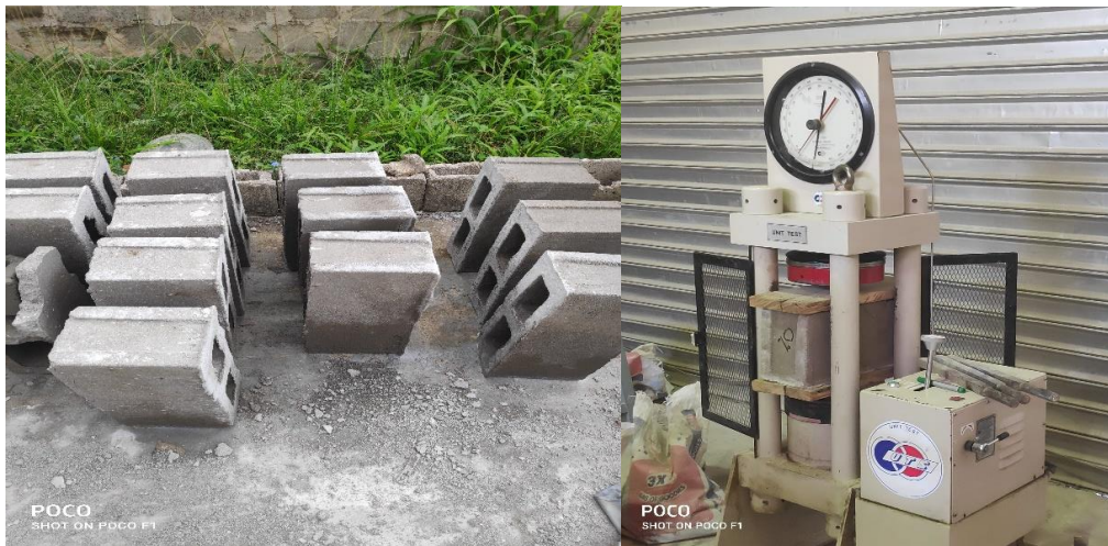
Figure 2. Hollow sandcrete block after water sprinkling; and under compressive load
