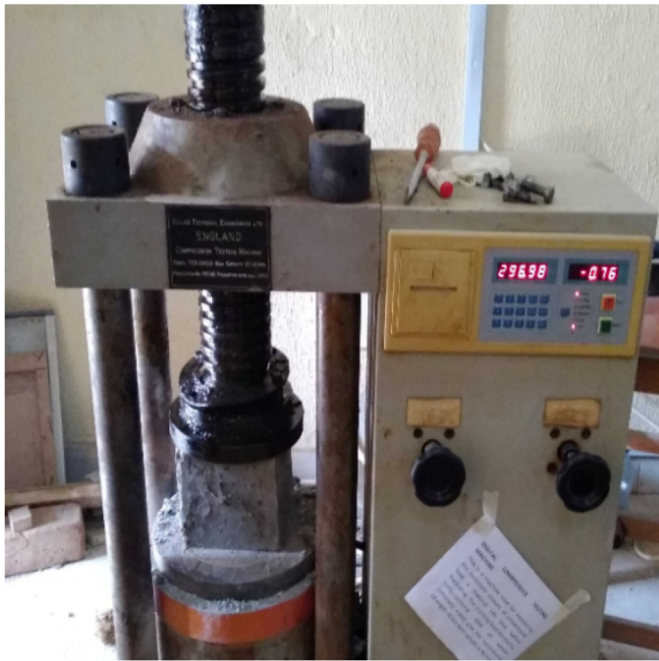
Fig. 3. Compression testing machine.
