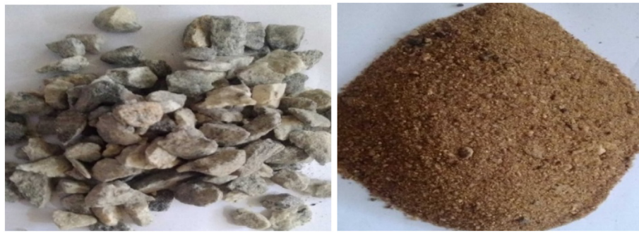
Fig. 1. (a) Granite (coarse aggregate); (b) River sand (fine aggregate).
