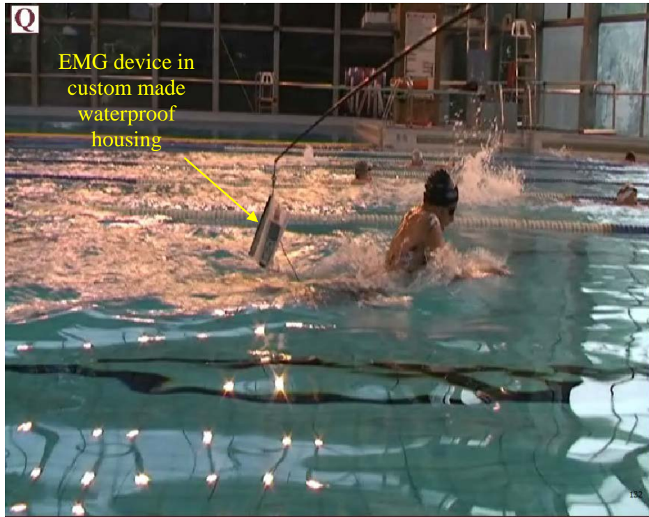
Plate 5.1 Shows a side view of the location of the EMG device in its waterproof housing and its location relative to the participant.
