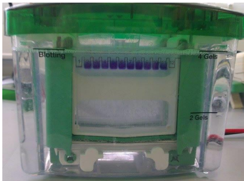
Figure 2.20: Photograph to show gel electrophoretic separation of homogenised adult rat ventricular tissue in sample buffer. As denoted by the pre-cast gels, wells were labelled 1-12 and the movement of the sample can be seen as the blue dye (sample buffer, containing protein) moving from the bottom of the wells.
