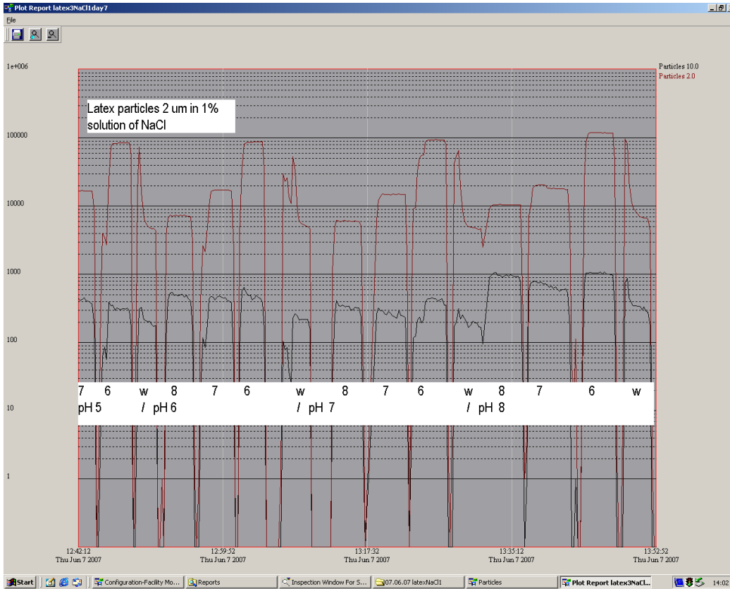
Figure 3 Latex particle size 2 \mu\text{m} in solution of 1% NaCl. Read by channel size 2, 5 \mu\text{m}
