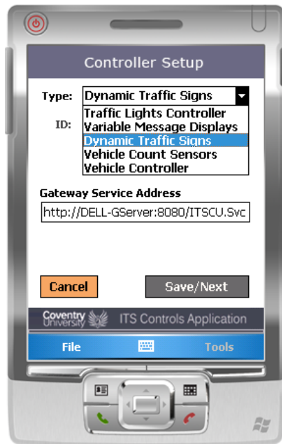
Figure 17: Controller Setup Screen – Select and Configure a traffic Controller type
