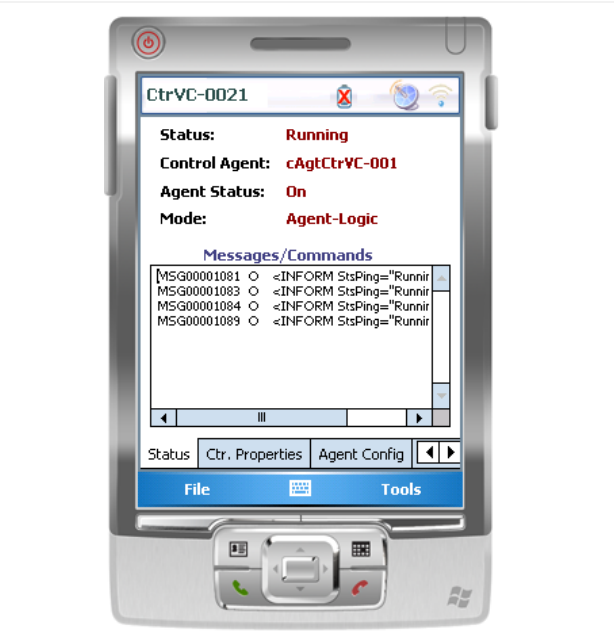
Figure 26: Controller Status Monitoring (Vehicle Count Sensor Controller Example)
