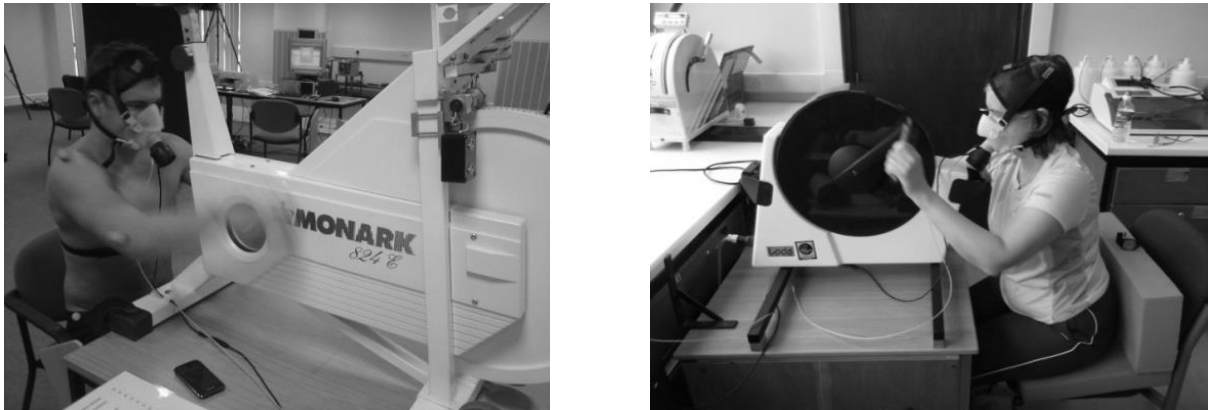
Figure 3.1: The upper body exercise set up for the modified cycle ergometer (left) used in study 1 and electronically braked arm crank ergometer (right) used in studies 2 & 4
