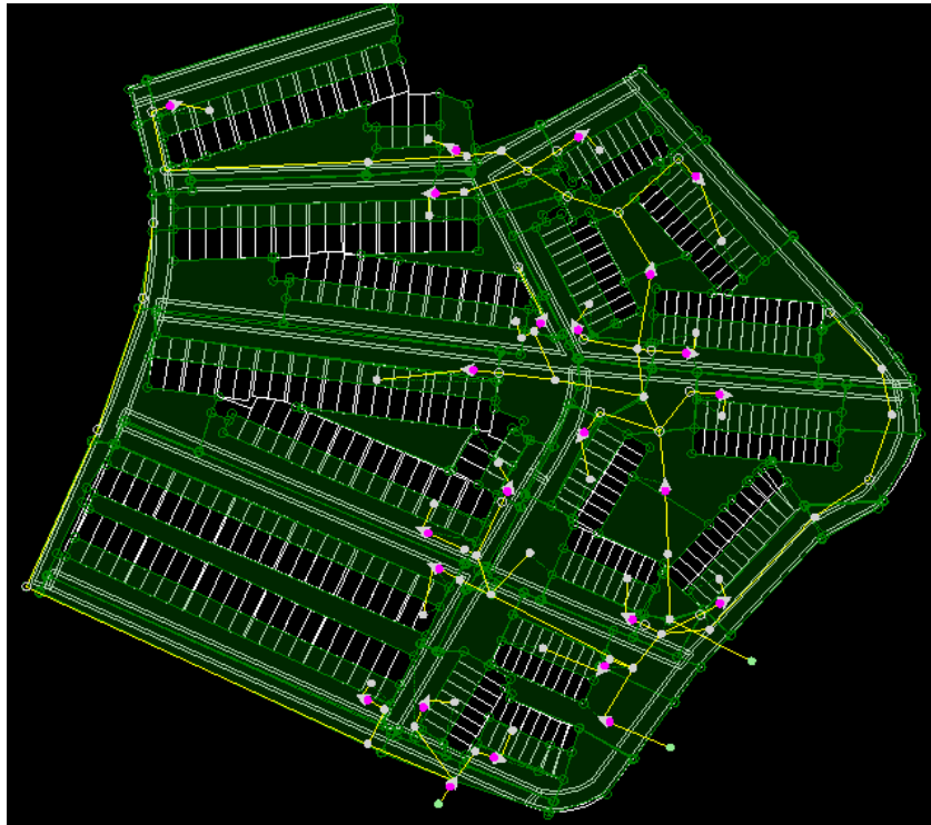
Figure 3-8 Designed SuDS Management train in MicroDrainage at Prior Deram Park, Coventry. Yellow lines are either pipes or swales, the triangles are either PPS or detention basins. Figure 3-7 for more detail.
