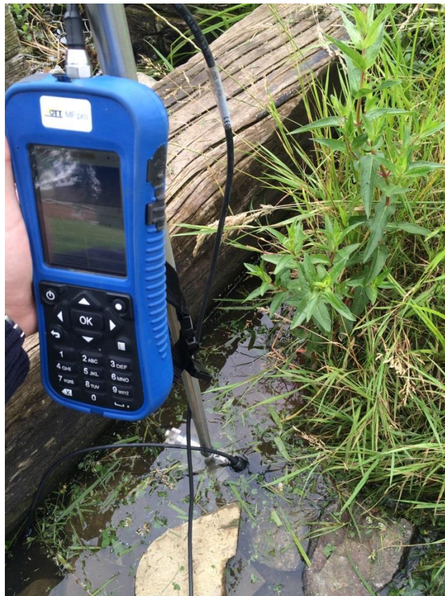
Figure 3-16 OTT MF Pro Spot Velocity Meter used at Hamilton, Leicester.
