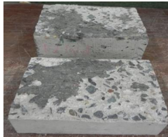
Figure 7-11 Tested prism saw-cut from tested composite beam of roughened OPCC interface: PMC patch bonded on OPCC interface
