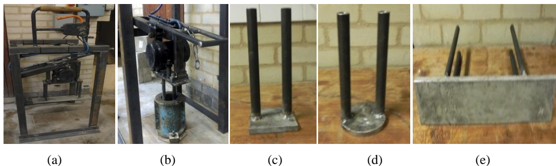
Figure 4-23 (a) vibrator and its components; (b) cylindrical specimen under compaction; (c) plate for blocks; (d) plate for cylinders; (e) plate for the formation of beams
