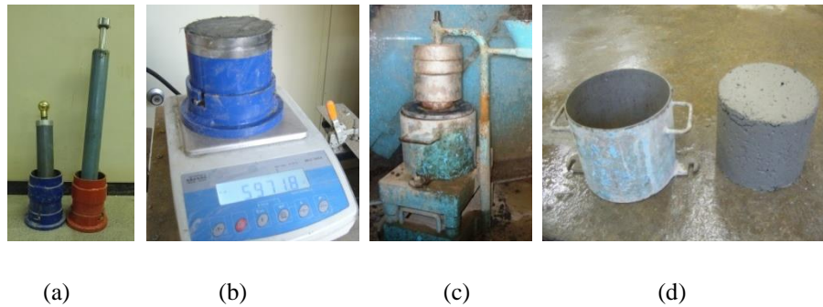
Figure 4-8 (a) devices for S-P(left) and M-P(right) methods, (b) compacted sample on balance, (c) M-VB tester, (d) container of M-VB and compacted sample by M-VB method
