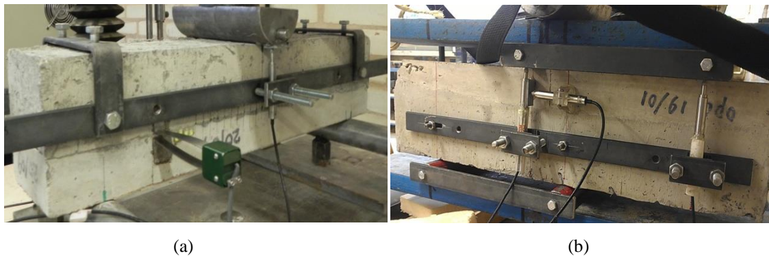
Figure 7-25 (a) experimental setup for SFRPMC-on-OPCC composite beam with interfacial notch under 3PB, (b) experimental setup for SFRPMC-on-OPCC composite beam with a notch through OPCC under shear test
