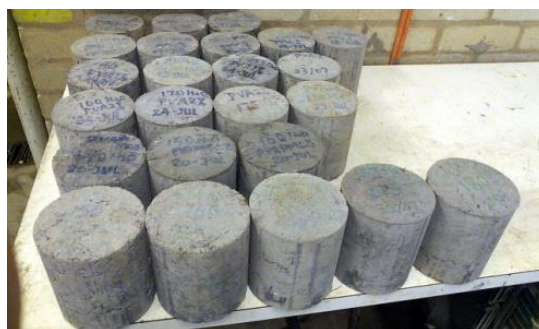
Figure 4-21 Six groups of compacted samples by M-L method for splitting tensile strength test (mixes M9 to M14 in Table 4-17 are in the order of front to rear)
