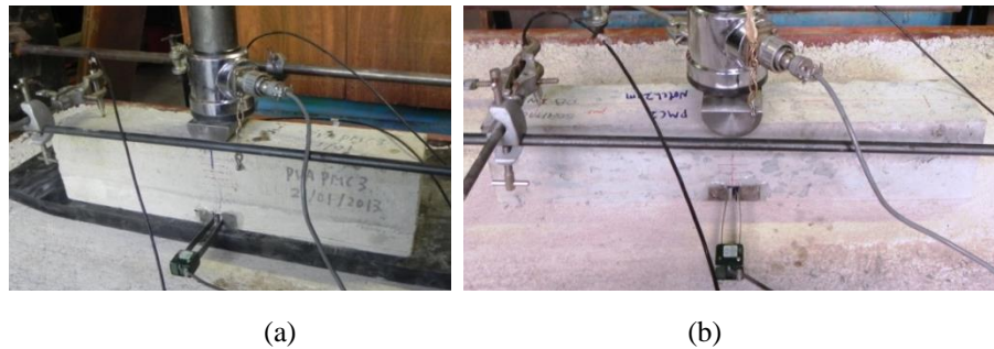
Figure 8-27 Experimental setup for SFRPMC-on-OPCC composite beam: (a) on RF, (b) on CF
