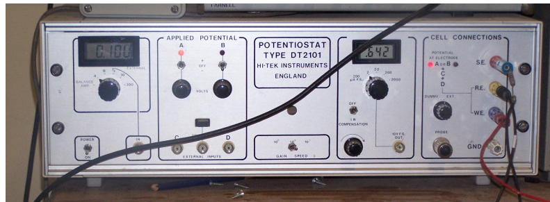
Figure 10-12 Potentiostat used to measure the polarization resistance in reinforced concrete samples
