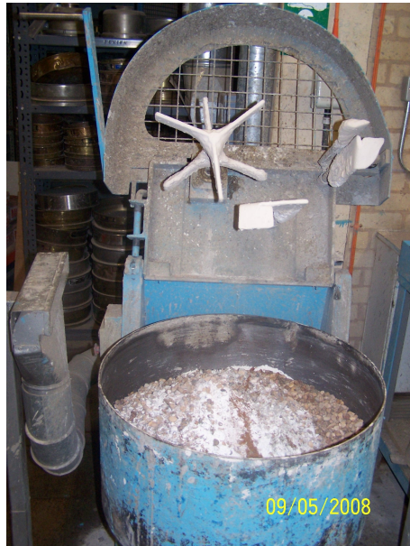
Figure 11-2 Horizontal 50 litre mixer
