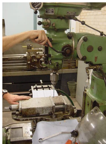
Figure 6-24 Vertical driller used for powder collection during a concrete chloride content analysis
