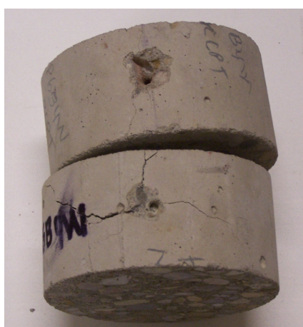
Figure 11-18 BPD sample cracked during drilling
