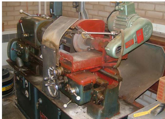
Figure 6-16 Machine used to cut concrete discs to be used in migration tests or porosity
