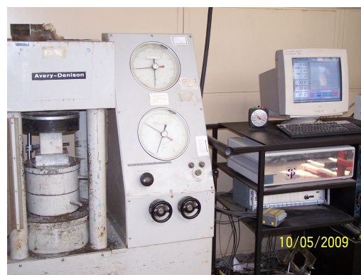
Figure 6-18 Cube crusher used to measure the compressive strength
