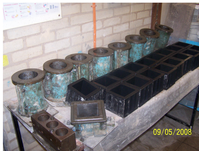
Figure 11-3 Pre-oiled moulds before casting
