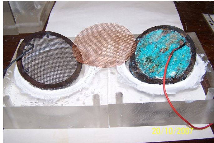
Figure 6-14 Copper electrodes used in migration tests; Left: cathode - centre: new mesh - right: anode
