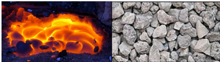
Figure 2-2 Blast furnace slag; left: molten slag – right: granulated slag
