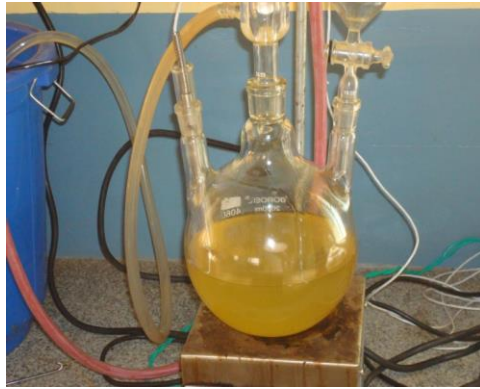
Figure 3. 9 One litre capacity esterification unit (Biofuel Park)
