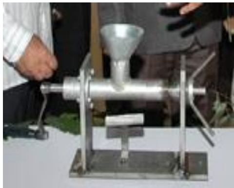
Figure 3. 8 Manually Operated Oil Expeller (Biofuel Park)
